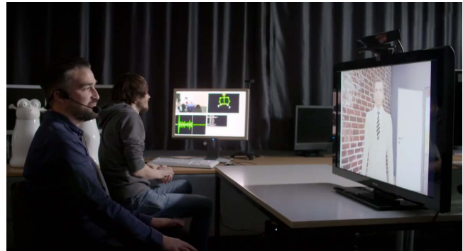
Figure 1: The PARLEY system including the Virtual Agent, the depth camera and the screen showing the open learner model.
